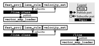
Fig. 1: Component-connector views of a publish-subscribe connector in Autoware.AI before (top) and after (bottom) a bug was introduced. Renaming the topic line\_class to line only in the publisher disconnected publishers and subscribers accidentally. The publishers and subscribers are dangling.
