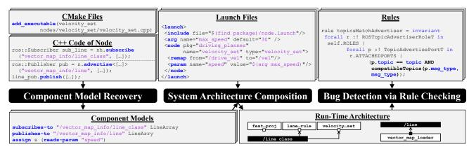
Fig. 2: Overview of the analysis stages (dark rectangles), data (rectangles), and data flow (arrows) of ROSDiscover. First, the component interface models are inferred from source code. Then, these models are composed according to architectural configuration files. Finally the architecture is checked against well-formedness rules specified in first-order logic.
