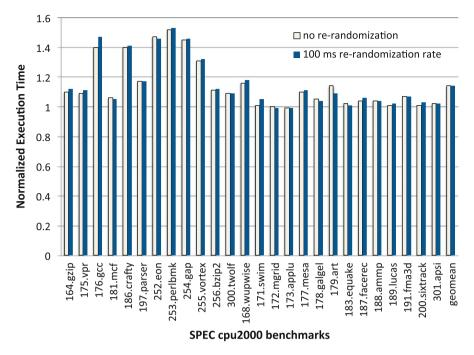
**Fig. 7.4** Performance overhead of dynamic ISR over native execution. Average performance overhead over native execution is 14%. Dynamic ISR at a 100 ms re-randomization rate adds virtually no overhead to the performance of running the Strata virtual machine
