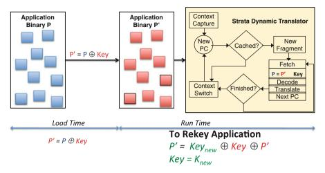
**Fig. 7.3** Dynamic ISR Implementation. At load-time, the program text is encrypted using an XOR key. The Strata VM is augmented with a decryption module that reapplies the key to recover the original program text. Throughout program execution, the program text is re-encrypted under a new key resulting in a dynamically shifting attack surface
