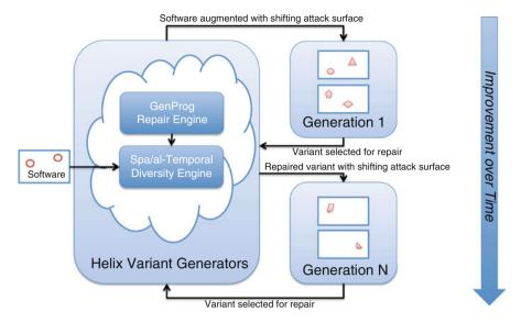
**Fig. 7.1** Helix Metamorphic Shield Architecture. Every software generation is augmented with a continuously shifting attack surface using spatial-temporal diversity transformations. Over time, via its GenProg component, Helix automatically reduces the attack surface by automatically generating and vetting candidate repair patches
